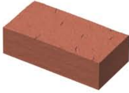
brique F pleine solid brick ladrillo M macizo Vollziegel M mattono M pieno
